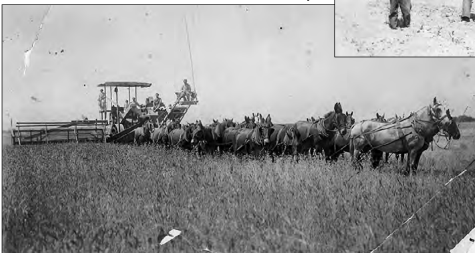
1914, Buttonwillow, California (Central Valley). Horse/mule-powered combine grain harvester, the Miller and Lux company.
