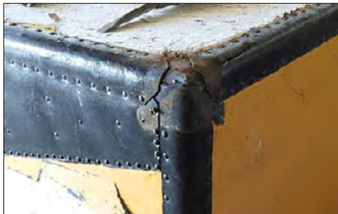
Corner showing trim, nails, finish (orange piece) and layer of cardboard under finish
