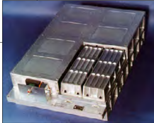
Guidance system computer. 16,000 word memory, 8 bit logic—Octal, 2,000 words programmable, required external cooling.
