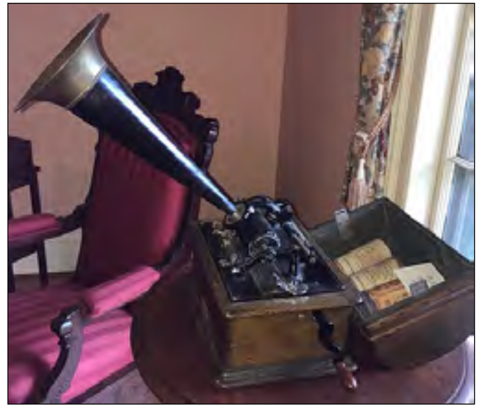
Ediphone, a sound recording device developed by Thomas A. Edison.
